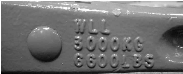
Indicator of Working Load Limit
