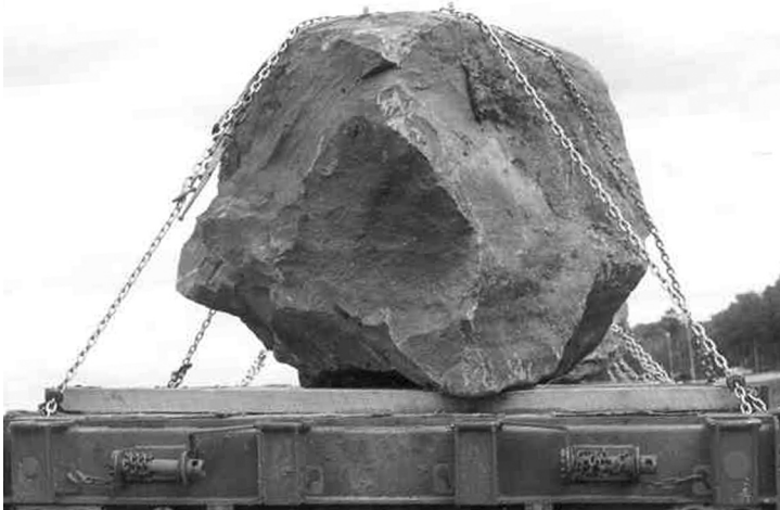
Chain is used to secure large boulders
